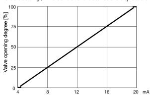
During initialization, the 1441 cPos-X positioner automatically detects the control function of the valve and is adjusted by default so that the valve is closed when the signal is 4 mA\*.
